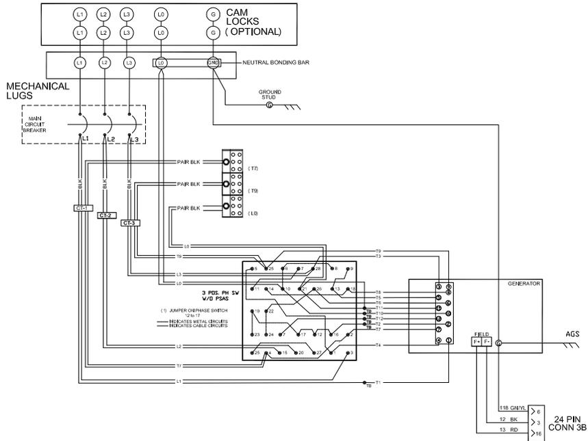
WIRING DIAGRAM FOR MDG175DF4 WITH 4 POSITION PHASE SWITCH EQUIPPED
