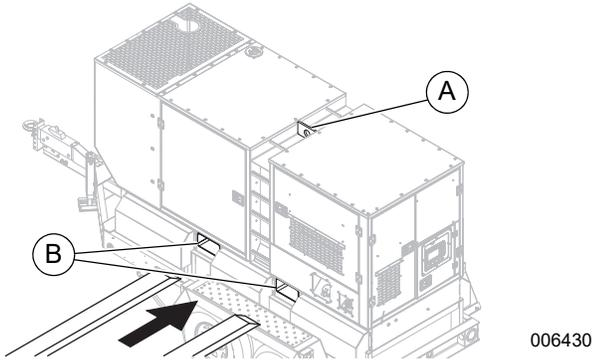
**Figure 3-14. Lifting Points**
