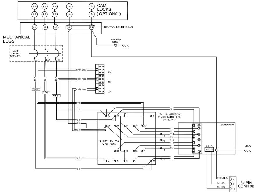
WIRING DIAGRAM FOR MDG250DF4 WITH 4 POSITION PHASE SWITCH EQUIPPED
