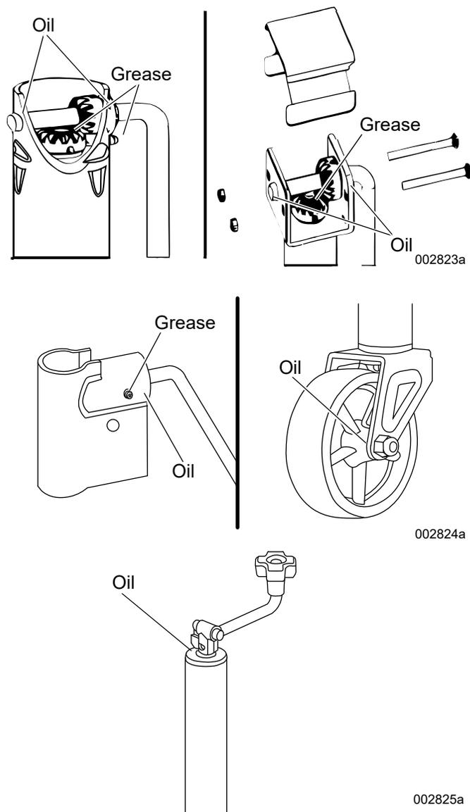
Figure 4-1. Lubrication Points
