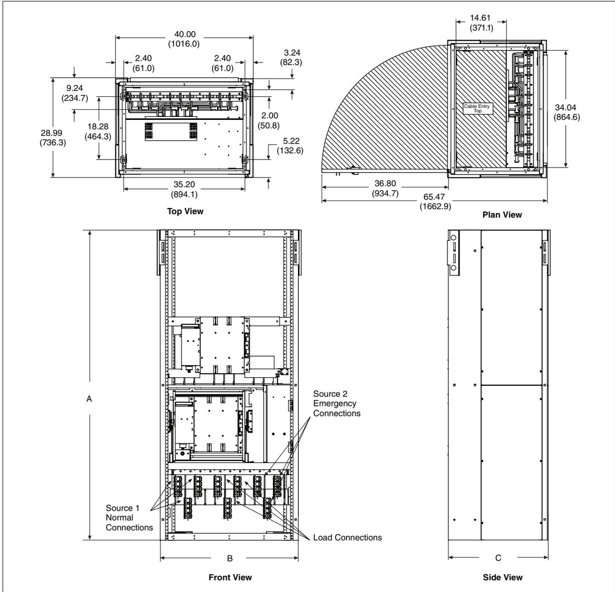
**Bypass Isolation Contactor NEMA 1 and NEMA 3R**
